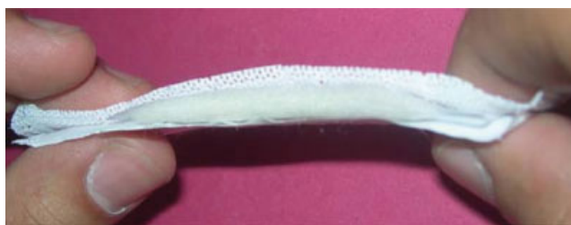
Figure 4 Cross sectional view of napkin with developed absorbent core. [Color figure can be viewed in the online issue, which is available at www.interscience.wiley.com .]
